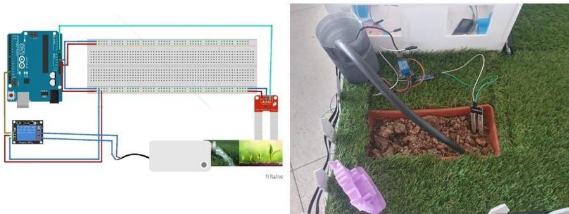
Figure 22. Simulation of the circuit using fritzing software and actual automatic watering system
