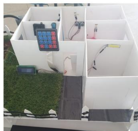
Figure 21. Simulation of the circuit using fritzing software and actual door security system
