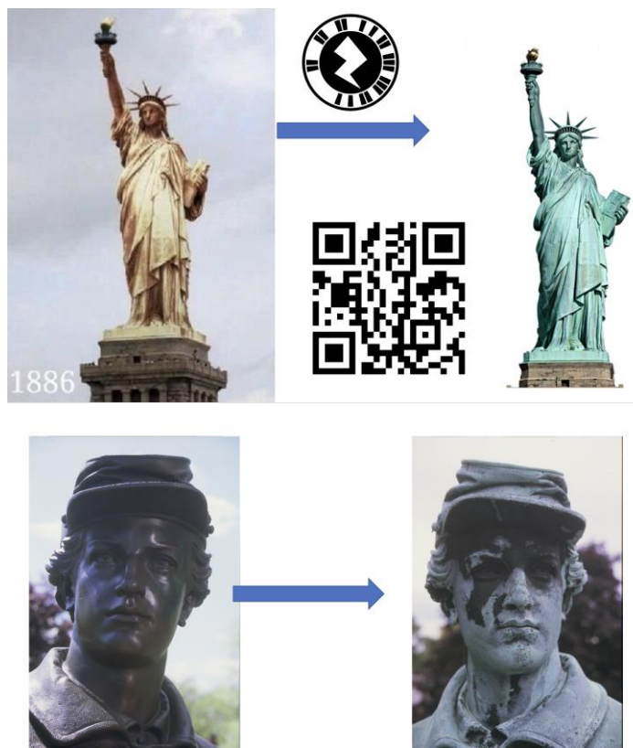
Picture 6. Two examples of metal corrosion in public monuments in the augmented reality application
