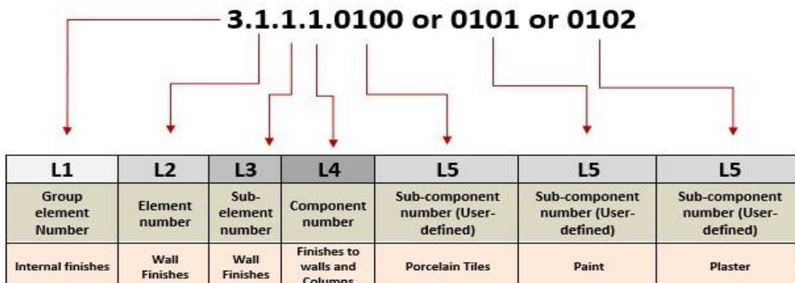
Fig. 8 Combination of 5 levels in NRM1- Column
