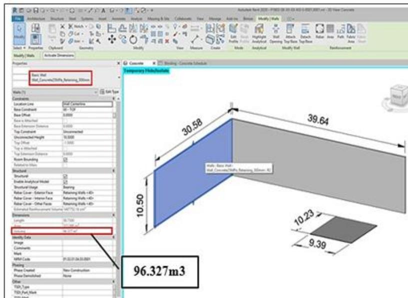
Figure 12. Total Quantity of Blinding Foundation
