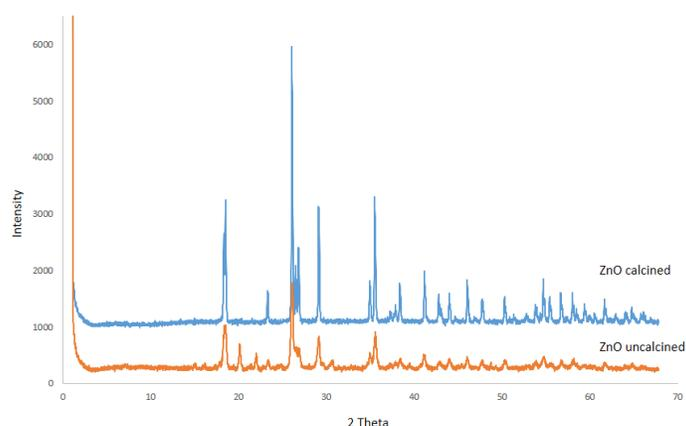
Fig 1. XRD of a. ZnO uncalcined and b. ZnO calcined.
