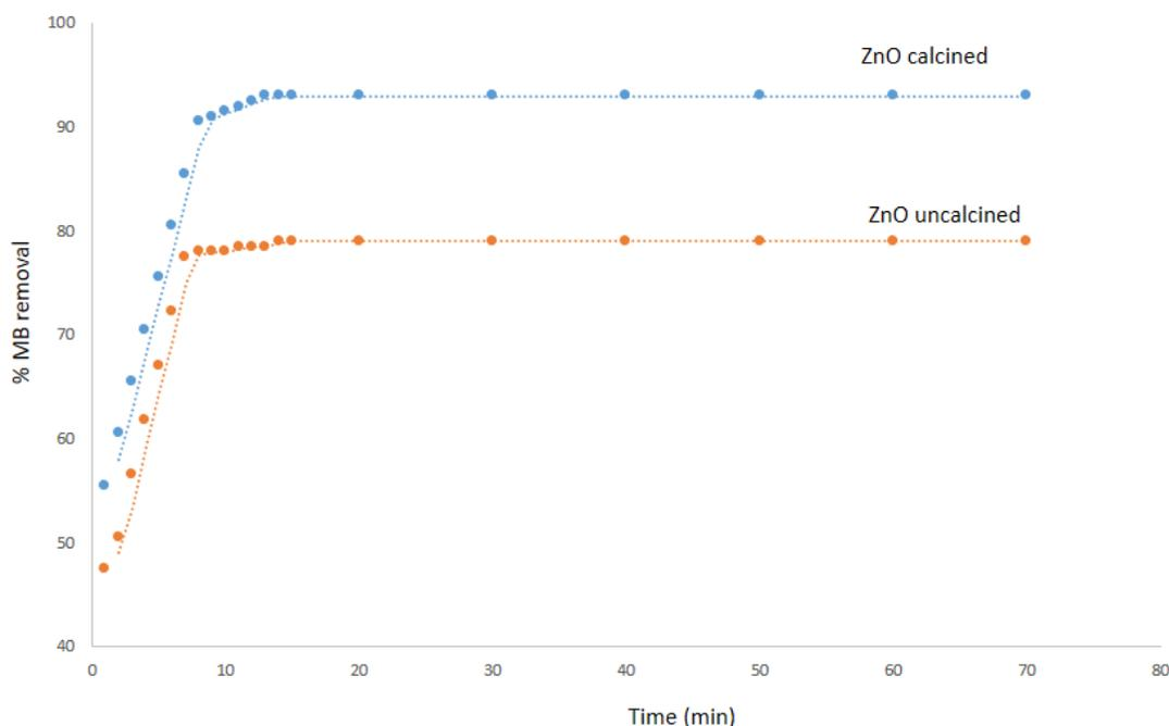
Fig 4. methylene blue Removal by Adsorption using ZnO calcined and ZnO uncalcined
