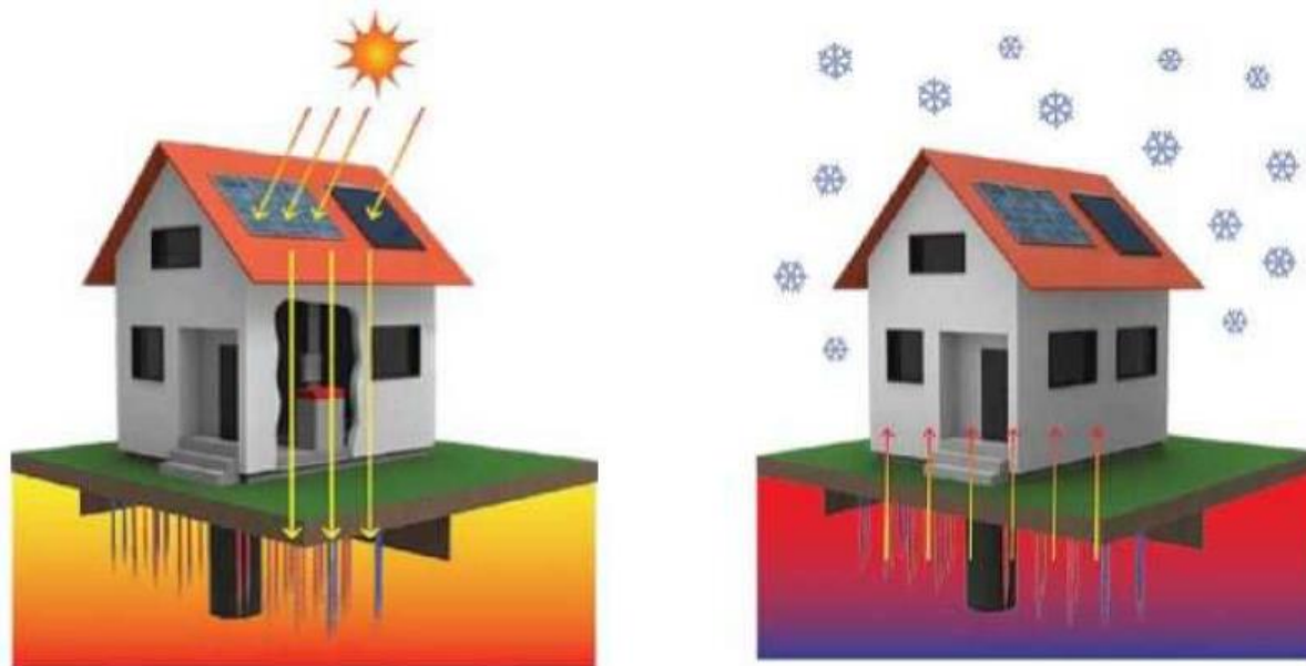
Figure 1: Operation of the earth energy storage system in summer and winter mode.
