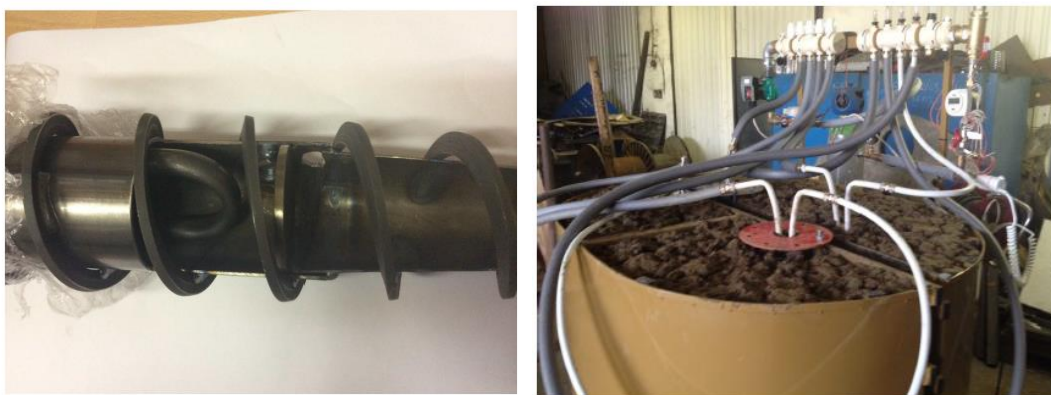
Figure 2: Testing of transport of thermal energy to geological subsoil in laboratory conditions by means of energetic needles.
