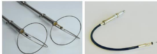
Figure 1: The draft probe, robust velocity temperature probe and manikin version
