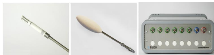
Figure 2: Humidity probe, operative temperature probe and main frame
