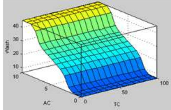
It can be clearly seen from figure 10.a, washing time isn't affected much by the amount of dirtiness. While, from figures 10.b, that the amount of clothes has a much higher affect in washing time than the type of clothes.
