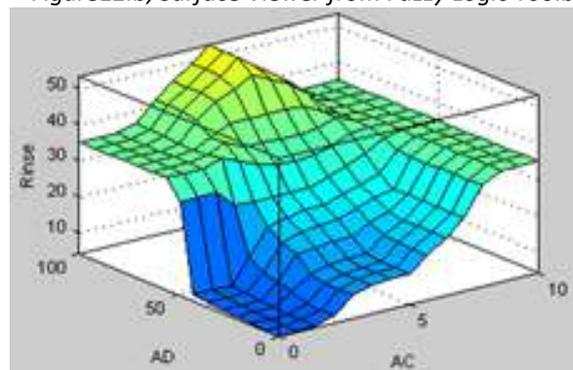
Figures 12.a and 12.b show the amount of both dirt and clothes are the most important factors which regulate the rinsing time. Whereas, the amount of clothes is directly proportional to the rinse time compared with amount of dirtiness. Figures below show the way the machine will response in different conditions. As sensors sense the input values and using the proposed system , the response of sensors are fuzzyfied and then by using if-else
