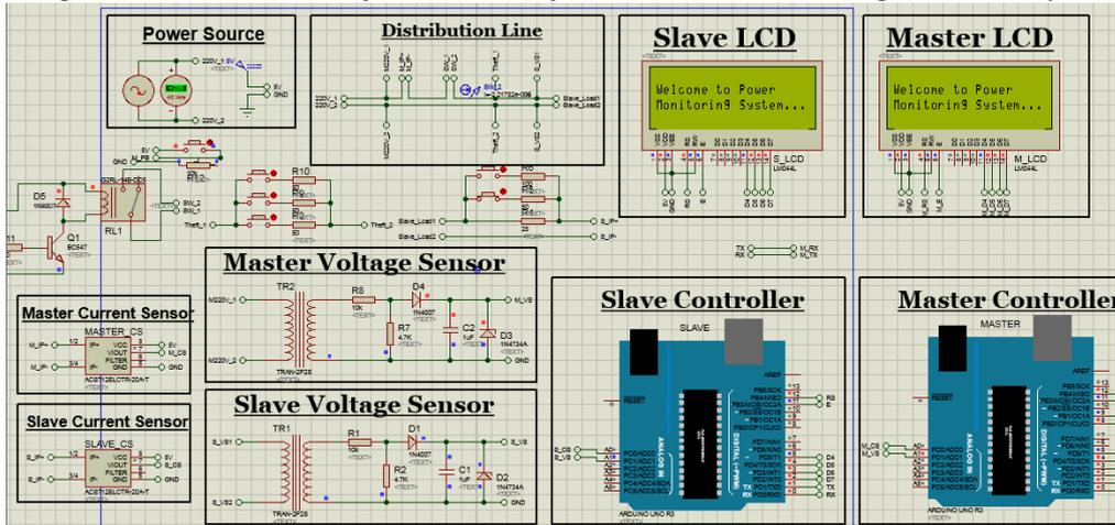
In the proposed system there are two three resistors, one of them, titled R4 = 25 ohm to represent the normal load and the two other resistor for representing the excessive power usage with two different quantities of load as shown in next figure.
