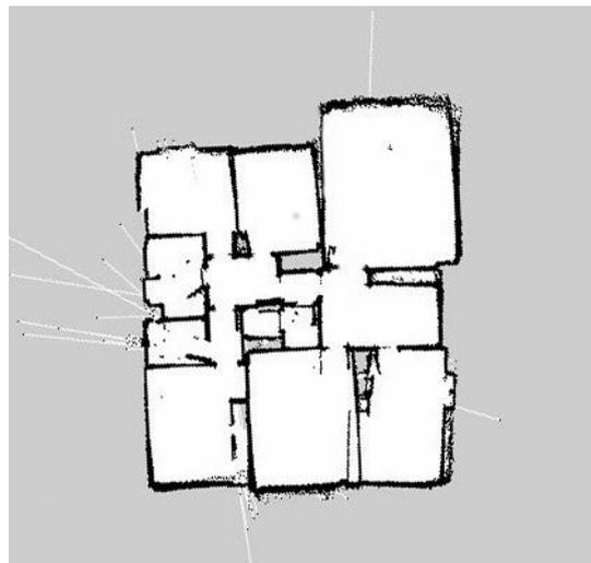
**Fig.6.** Mapping with LIDAR
