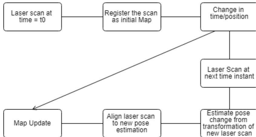
**Fig.5.** General Flow Diagram
