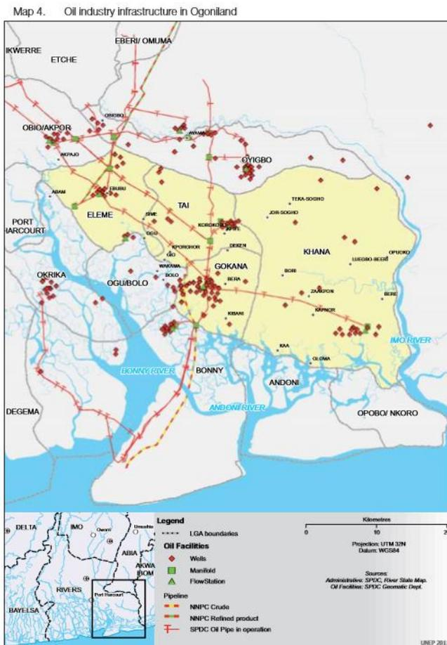
Fig. 3. Oil Industry Infrastructure in Ogoni (including the Trans Niger Pipeline)
