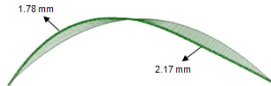
Figure 9. FE: Deformed shape of the parabolic arch for L:h = 4 ; load case A2
