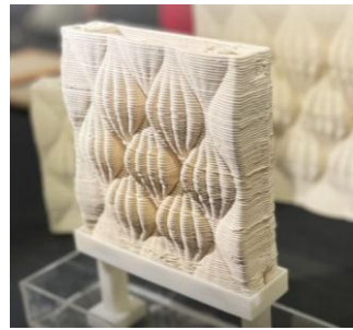
Figure 3: Klimatile prototype cladding system ceramic tile
